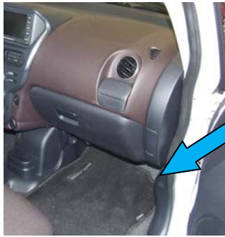
The hood release is under the instrument panel beside the front passenger's door.
